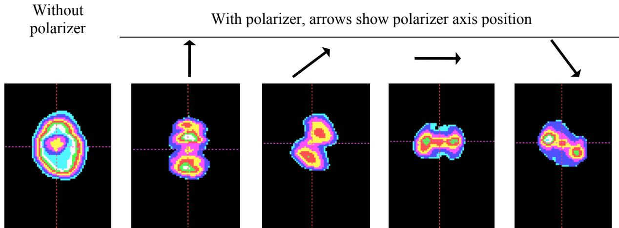
Fig.4. Diagnostics of a radially polarized beam. The arrow shows positions of the polarizer axis.
