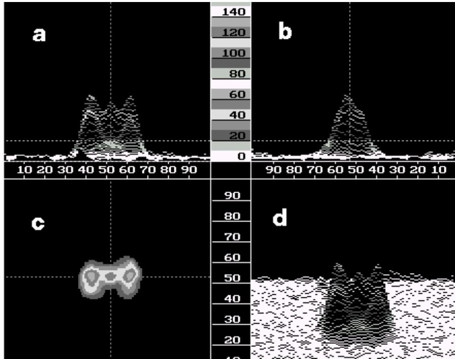
Fig.3. A typical picture of intensity distribution of the laser beam transmitted through the polarizer obtained with MAC-2. The axis of the polarizer is directed a flat in the picture c.
