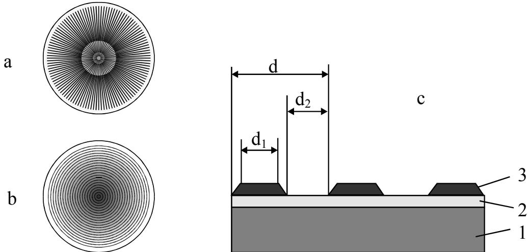
Fig.2. The structure of grooves of the optical elements for generating radially (a) and azimuthally (b) polarized radiation. The structure of the optical element (c): silicon substrate 1, adhesion Ti-layer 2, relief Cu-layer 3.
