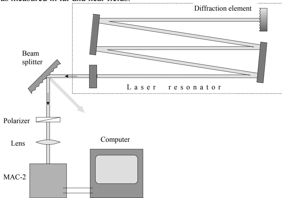
Fig.1. The optical scheme of the experimental setup.
