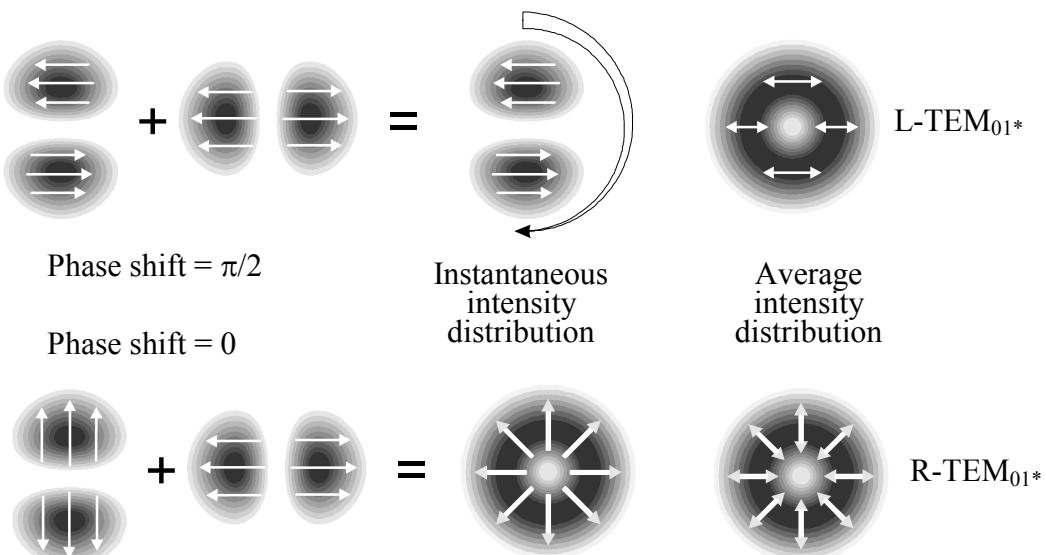
Fig.6. Formation of the radially and linearly polarized modes with ring intensity distribution.
