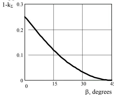
Fig.8. Dependence of losses of the “compound” mode TEM<sub>01\*</sub> formed by two plane polarized modes TEM01 with the angle shift 2β.
