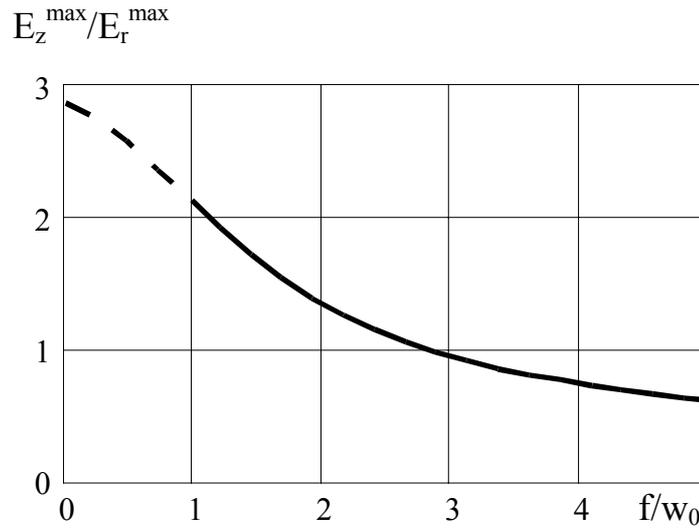
Fig. 4. The ratio of maximum amplitudes of longitudinal and transverse electrical fields in the focal plane versus the focal length in Debye approximation.
