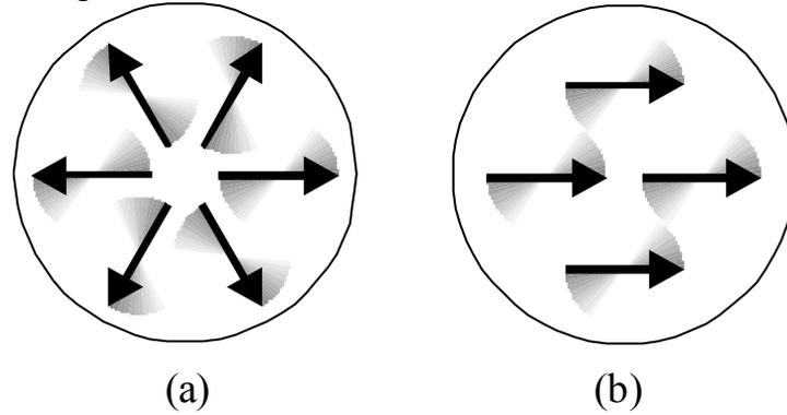
Fig. 2. The helical (a) and conventional (b) modes with circular polarization. Arrows show instant direction of electric vector and distribution of its phase over the cross-section. The tail area of the arrows shows direction of rotation.
