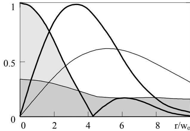
Fig. 5. The illustration of relative distribution of  $E_z$  (filled regions) and  $E_r$  (curves) at the waist  $z=0$  (thick lines) and at the distance  $z=8w_0$  (thin lines). The focal distance is  $f=2.6w_0$ . The scale of all curves is the same.
