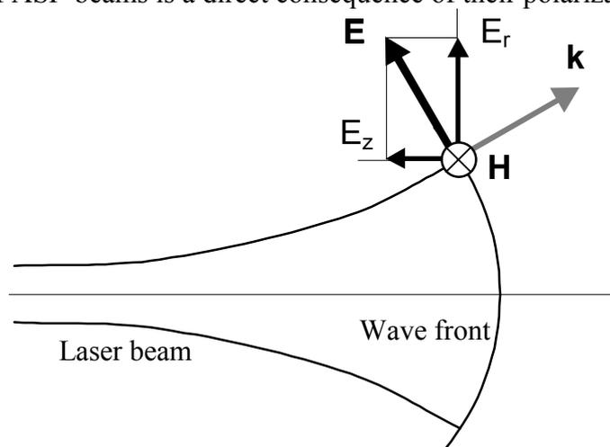
Fig. 1. Schematic view of relative location of the electromagnetic field and the wave vector  $\mathbf{k}$  for a beam with r-z directed field.
