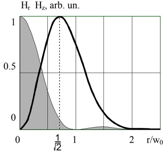
Fig. 3. Radial distribution of longitudinal components  $H_z$  (filled region) and radial  $H_r$  (curve), obtained from (5).
