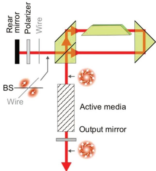
Fig. 7. (Color online) Schematic of use of a Sagnac interferometer in a laser resonator as a rear mirror to generate inhomogeneously polarized modes.
