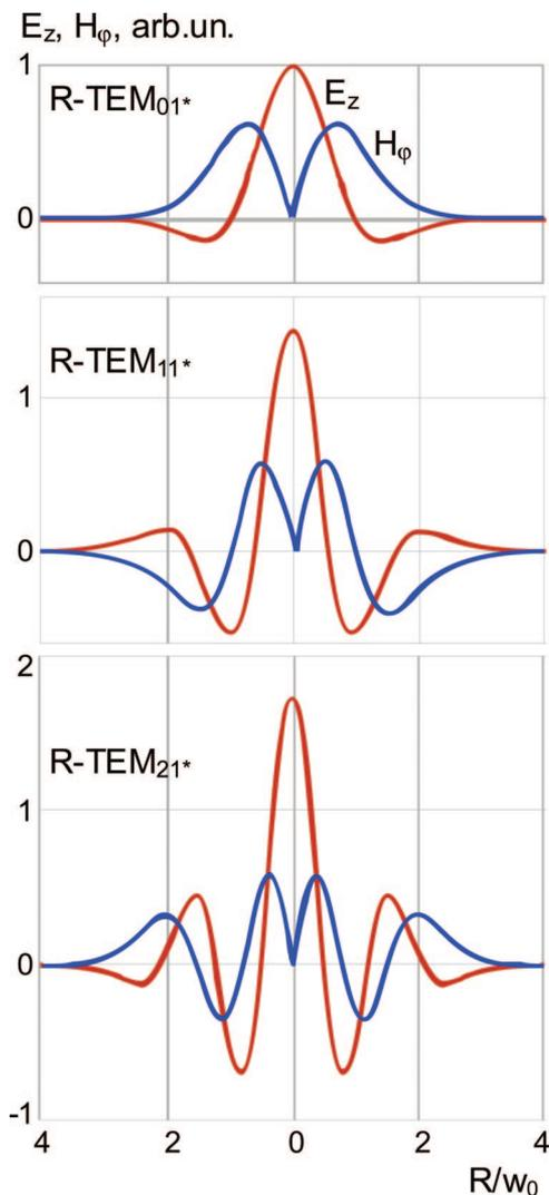
Fig. 9. (Color online) Calculated distributions of longitudinal components of electric field  $E_z$  and azimuthally directed magnetic field  $H_\phi$  in the waist for the radially polarized modes of different orders.
