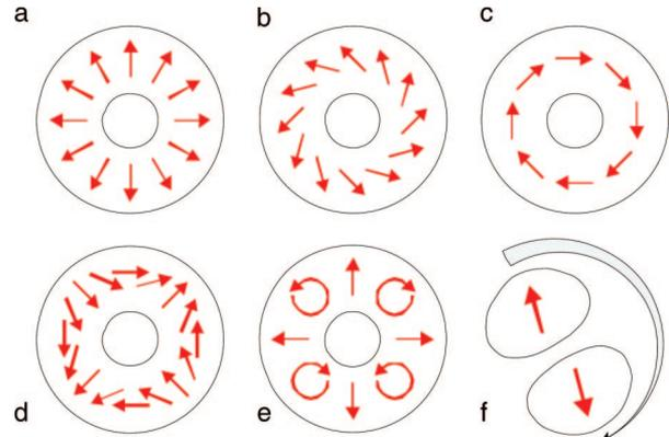
Fig. 4. (Color online) Examples of inhomogeneously polarized resonator modes. (a) Radially polarized mode  $R\text{-TEM}_{01^*}$ . (b) The angle between  $\mathbf{E}$  and radius is  $45^\circ$ . (c) Azimuthally polarized mode  $A\text{-TEM}_{01^*}$ . (d) The mode with different directions of electric field. (e) The mode with different types of polarization. (f) Helical mode with plane polarization.
