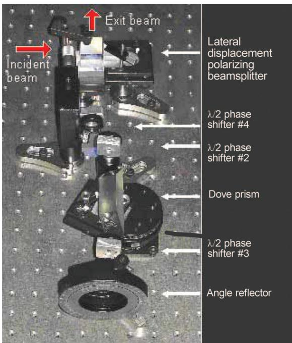
Fig. 3. (Color online) Modernized Sagnac interferometer mounting on an optical table.
