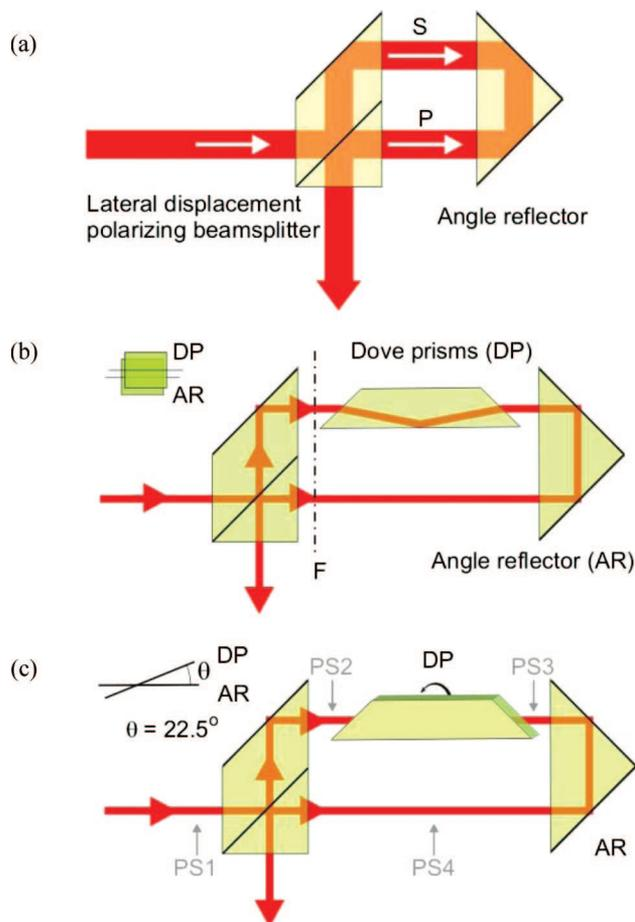
Fig. 1. (Color online) Schematic of a Sagnac interferometer. (a) Simplified schematic; P and S are the corresponding polarization of two beams. (b) Schematic with a Dove prism. (c) Modified Sagnac interferometer configuration to produce laser beams with inhomogeneous polarization.
