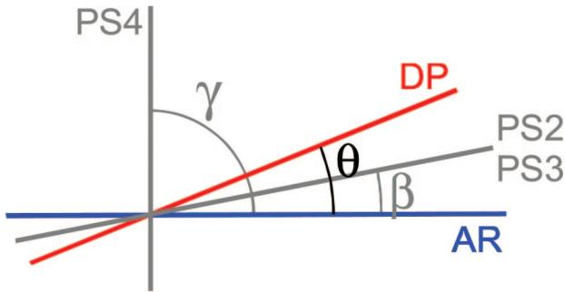
Fig. 2. (Color online) Graphical explanation concerning installation of half-wavelength phase shifters into experimental setup, where  $\beta = 10.25^\circ$ ,  $\gamma = 90^\circ$ , and  $\theta = 22.5^\circ$ .
