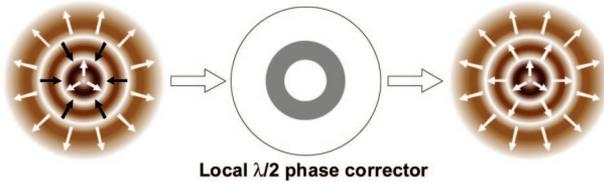
Fig. 8. (Color online) Phase correction of the high-order radially polarized mode.
