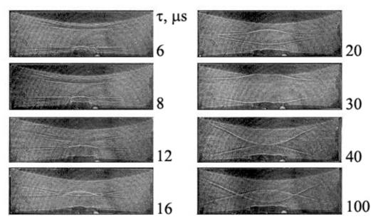
Schlieren pictures of the shock waves traveling from electrodes opposite each other. The pictures were made after pulsed discharge in carbon dioxide. The waves cross each other and reflect from the electrodes. Discharge pulse duration is  $\sim 1 \mu s$ . Duration of exposition is 30 ns. The delay time of exposition after discharge is from 6 up to 100  $\mu s$ .
