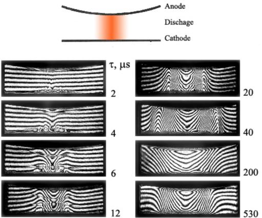
Interferograms of gas dynamic disturbances in discharge gap obtained after pulsed discharge in cabon dioxide. Gas pressure is 100 Torr. Discharge pulse duration is  $\sim 1 \mu s$ . Duration of exposition is 30 ns. The delay time of exposition after discharge is from 2 up to 530  $\mu s$ .
